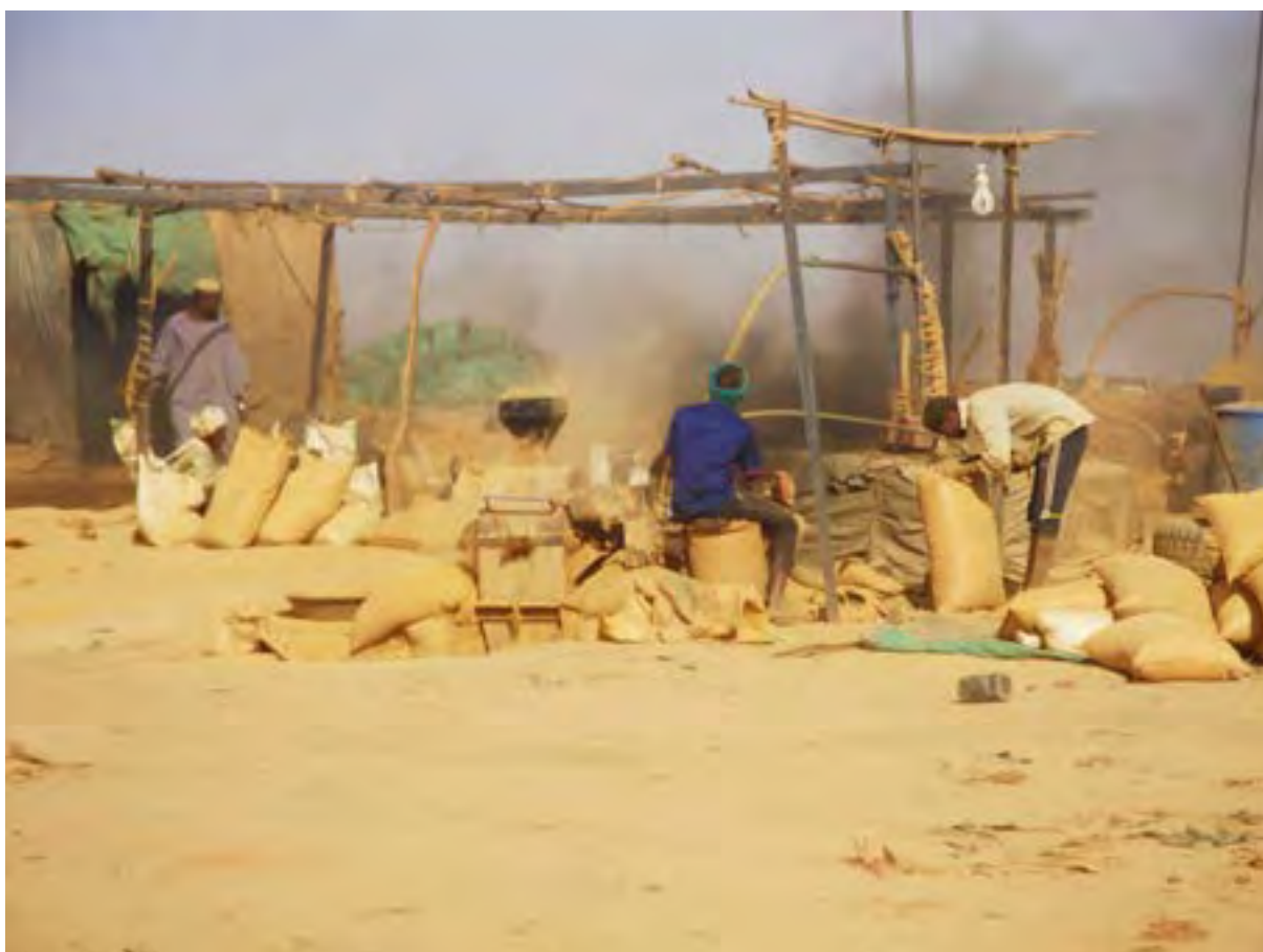
Grinding of crushed rocks by artisanal miners causes a dual hazard from dust and grinder's exhaust. Photo credit © Osman Ali
